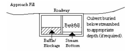
c. Culverts shall be designed and installed in such a manner that the original stream profiles are not altered and allow for aquatic life movement during low flows. The dimension, pattern, and profile of the stream above and below a pipe or culvert shall not be modified by widening the stream channel or by reducing the depth of the stream in connection with the construction activity. The width, height, and gradient of a proposed
